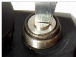
J-3 Use a flat head screwdriver to adjust the windage and elevation.
