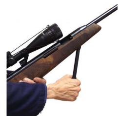
cocking stroke. This safety device gives additional security when inserting a pellet, however the user is still advised to keep hold of the cocking arm as illustrated above. Be sure that you do not obstruct the safety catch button and prevent it from working during the cocking process.
