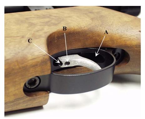
Remember that small adjustments will make a noticeable change to the operation of the trigger. Only make 1/4 turn adjustments at a time and test fire the rifle before making further adjustments. Jot down all adjustments on a piece of paper so that you can retrace your steps if necessary.
