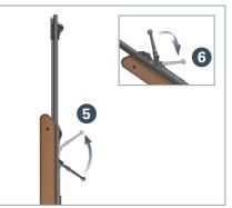
**4**. Close and lock the bolt by pushing the bolt handle up **5** and right **6**.
