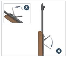
**3**. Pull the bolt handle left **3** and down as shown **4** to its open position until a click sound is heard.
