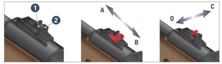
**Elevation adjustment:** Loosen screw **1**. If the point of impact is too low: adjust rear sight to **A** (front). If the point of impact is too high: adjust to **B** (back). Tighten screw **1**.
