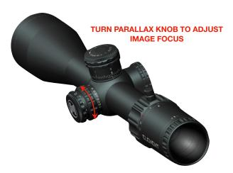
Tip: Place your riflescope in a fixed position and change the position of your eye (up/down, left/right) while adjusting parallax. If parallax is not set correctly, there will be apparent movement of the reticle in relation to the target. Adjust the parallax until this movement is eliminated.
