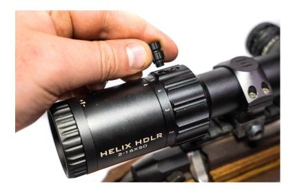
Your HELIX HDLR will need to be zeroed after it has been fitted to your rifle. The Elevation & Windage turrets feature different designs, and need to be reset differently. The first step is to lift the elevation turret housing and remove the zero stop mechanism to allow a full range of adjustment.
