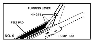
CAUTION: Improper lubricants, such as aerosol type spray lubricants, can ignite (diesel) during pumping. Use only automotive motor oils.
