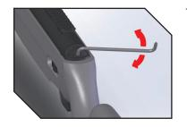
TRIGGER WEIGHT ADJUSTMENT: The factory setting for the trigger weight is 3 lbs. The trigger weight can be adjusted in 2 oz increments from a minimum of 2.5 lbs to a maximum of 3.5 lbs. The trigger weight adjustments are made by turning the embedded screw behind the receiver using either the included tool, or a #1 Philips screwdriver.
