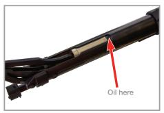
It is also recommended to lubricate the pump arm linkage and bolt pivot points with machine oil every six months.
