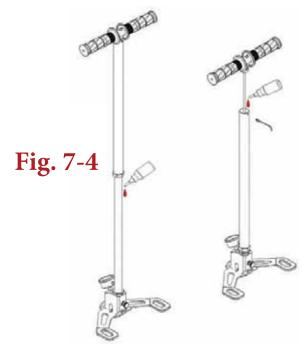
Lubricate pump with silicone oil as shown.
