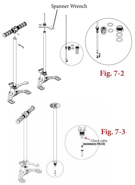
Using the spanner wrench, open the check valve in the base plate. Clean or replace the check valve.
