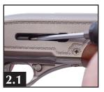
3 - Insert the cocking bolt and line up the screw hole in the bolt with the screw hole in the hammer. With the included allen key, install the allen head screw. Tighten securely.
