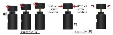
**3:** To remove the UFA knob, ensure thwe 8/32 set screws are loosened and turn the UFA knob (**part 2**) counter clockwise towards the "closed" position until the UFA knob is fully removed from the UFA pin as shown in **example:** (**C**).
