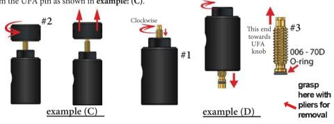
**4:** To remove the UFA pin (part 3) from the UFA body (part 1), screw the UFA pin CLOCKWISE into the UFA body from the top portion of the UFA until the UFA pin comes out of the bottom of the UFA body (as shown in example (D)).
