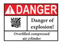
Do NOT exceed <u>maximum fill</u> <u>pressure of 310 bar/4,500 psi at</u> room temperature!
