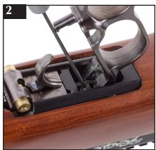
A WARNING: THIS ADJUSTMENT AFFECTS SEAR ENGAGEMENT. DO NOT OVER-ADJUST, AS THIS MAY CAUSE THE AIRGUN TO FIRE PREMATURELY OR NOT OPERATE CORRECTLY AND MAKE THE AIRGUN UNSAFE. ALWAYS CHECK YOUR SETTINGS TO ENSURE CORRECT AND SAFE OPERATION OF THE AIRGUN. ALWAYS ENSURE THAT OPERATION OF THE SAFETY IS UNAFFECTED BY ANY ALTERATIONS YOU MAKE TO THE TRIGGER MECHANISM.
