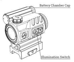
The illumination is powered by a AAA battery. Remove the battery chamber cap by turning it counter-clockwise and then set the battery with the positive (+) side facing in. Reinstall the cap by turning it clockwise, DO NOT OVER TIGHTEN.
