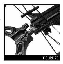
4. Carefully seat the riser into the mounting area on the arrow/flight track. Ensure the cables are properly placed in the fore-end cable track and the string lies above the arrow/flight track.
