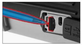
To remove the microSD Card from the slot, push it in using the same thin object. When it pops up a few millimeters, it can be pulled with your fingers or tweezers.
