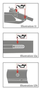
al parts (receiver, screw heads, trigger, etc.) are a gun blue finish and MUST be wiped clean using a slightly oiled cloth after handling to prevent rust. Use light acid free and resin free oil.
