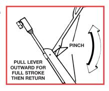
CAUTION: Be sure to grasp pump handle firmly as you close the lever to prevent it from snapping back and causing possible injury. Also be careful to keep fingers out of cocking mechanism when closing lever. (See "PINCH POINTS," Drawing No. 2).
