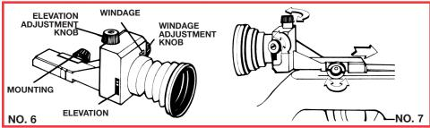
**Installation:** Mounting is accomplished on the dovetailed receiver of the Avanti Elite, model 753, Competition Pellet Rifle by loosening the mounting screw and plate, and sliding the sight onto the dovetail grooves of the receiver. Position sight where you want it in relation to your eyesight and/or physique. Tighten mounting screw securely.
