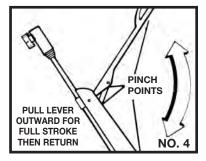
**CAUTION:** Be sure to grasp pump handle firmly as you close the lever to prevent it from snapping back and causing possible injury. Also be careful to keep fingers out of cocking mechanism when closing lever. (See "PINCH POINTS," Drawing No. 4).
