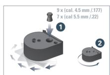
2. Insert the pellet as shown into the magazine 1 and slightly turn the plate to the next pellet chamber. Repeat until all pellet chambers are filled, then turn the plate back to its original position 2.
