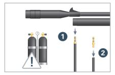
4. Scuba tank: BLEED the fill hose COM-PLETELY before disconnecting the quick-fill adapter from the air pistol to avoid hose whip and possible injury.
