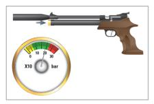
3. Watch the gauge on the air pistol and charging equipment. We recommend to fill the tank with a pressure of 200 bar. **Do not exceed a filling pressure of 200 bar!**
