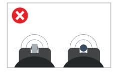
**Elevation adjustment:** If the point of impact is too high: turn screw **1** clockwise. If the point of impact is too low: turn screw **1** counterclockwise.
