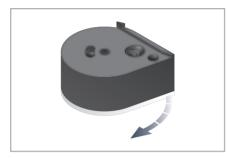
**1.** Hold the magazine (as shown) and rotate the transparent plate until the first pellet chamber becomes visible in the loading aperture.
