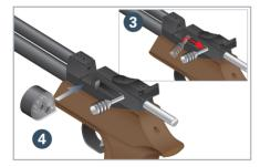
**3**. Pull the bolt handle backward to its open position **3** until a click sound is heard. Now insert the loaded magazine as shown **4**.
