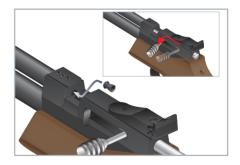
2. Insert a pellet (as shown) flush into the barrel and close and lock the bolt by pushing the bolt handle forward and down. **Do not** fill in more than 1 pellet.
