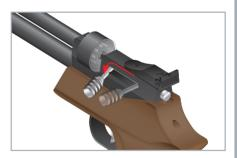
4. Close and lock the bolt by pushing the bolt handle forward and down. Do not load more than 1 pellet into the barrel. Immediate shooting after cocking is recommended to prevent loading of 2 pellets into the barrel.
