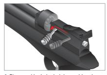
**4.** Close and lock the bolt by pushing the bolt handle forward and down.
