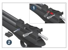
1. Pull the bolt handle backward to its open position 1 until a click sound is heard. Now insert the loading base 2.
