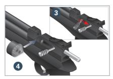
3. Pull the bolt handle backward to its open position 3 until a click sound is heard. Now insert the loaded magazine as shown 4.
