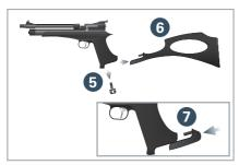
2. Detach the rifle's stock screw 5 and remove the stock 6 by pulling it backwards. Slide the pistol's grip cap 7 onto the grip and re-tighten the stock screw.
