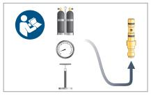
1. Read all instructions about your charging equipment and connect the quick-fill adapter to it. **Please note that** your charging equipment must include a pressure gauge (manometer)!
