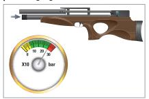
3. Watch the gauge on the air rifle and charging equipment. We recommend to fill the tank with a pressure of 250 bar. **Do not exceed a filling pressure of 250 bar!**
