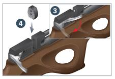
8. Pull the bolt handle backward to its open position 3 until a click sound is heard. Now insert the loaded magazine as shown 4.
