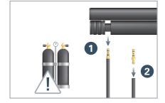
4. Scuba tank: BLEED the fill hose COMPLETELY before disconnecting the quick-fill adapter from the air rifle to avoid hose whip and possible injury. Disconnect the quick-fill adapter from the air rifle 1 and the charging equipment 2. To decock, aim in a safe direction and pull the trigger.
