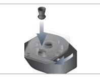
**6.** Turn the transparent plate clockwise to the next chamber and insert the next pellet.
