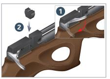
**1.** Pull the bolt handle backward to its open position **1** until a click sound is heard. Now insert the loading base **2**.
