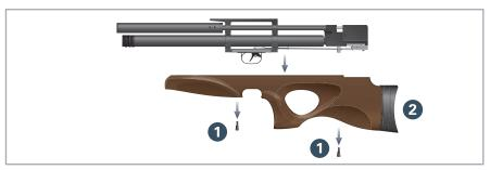
**1**. Loosen the stock screws **1** and remove the system from the stock **2**.
