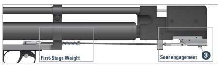
Note: Use a hexagon (Allen) key (SW 1.5) to adjust the trigger.
