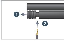
2. Ensure that both, fill adapter and filler, are clean from dirt. Pull back the protective cap and insert the fill adapter into the intake valve and start filling. If you use a scuba tank, fill **slowly** to prevent heat building.
