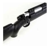
Hold the bolt handle continue to pull back until it locks in place. Do not lower the bolt handle. Push the bolt handle forward and lower to its original postion and it is ready to fire.
