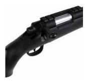
Lift up on the bolt handle from the end of the handle. Once the handle is up it is clear of the stock and able to be pulled backwards.
