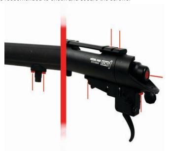
The highlighted locations are the check points on the M28. You can use a thread locking glue or Loctite to keep the screws in place over time. You only need to hand tighten the screws to secure them. Over tightening will cause damage.
