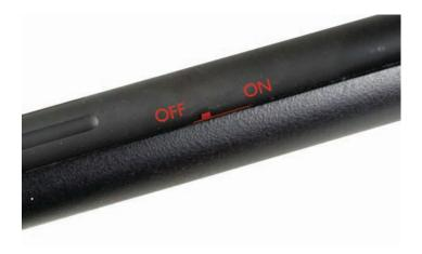
**Step 2.** Slide the hop up adjuster tab back towards the trigger to add more hop effect. Sliding forward will turn off the hop up unit.
