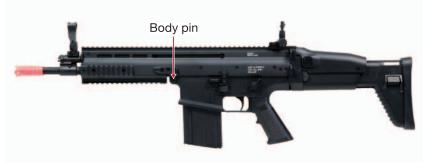
To drop the lower receiver press the body pin to the side. The body pin is held in the lower by a metal clip. Once the body pin is loose you are able to pivot from the rear and seperate the lower. Make sure the bolt and charging handle is forward for an easier procedure.
