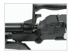
**Step 2.** Keep the outer barrel lock pressed in and pull the outer barrel forward. If the outer barrel is stuck please wiggle the outer barrel until free.
