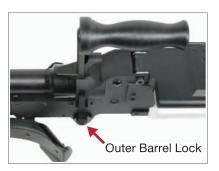
**Step 1.** Remove the heat shield. Press and hold the outer barrel lock and lift the carry handle up.
