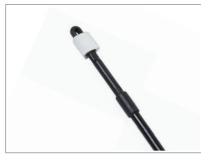
Cut the cloth or paper towel in the size as shown above. Fold the material to fit through the loop. Adjust the length of the material to smoothly enter the barrel. Otherwise too much material will get jammed in the inner barrel and can cause the hop up bucking to get out of place.
