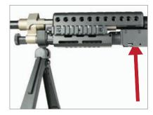
**Bipod 3.** Extend the bipod legs out and allow gun to rest. Press the bipod lock plate up to secure.
