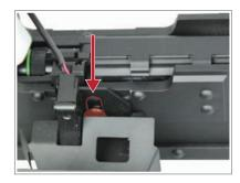
**Step 2.** Gently slide the magazine mount on and down. Make sure the thin power wire is up and out of the way to prevent it from getting pinched.
