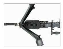
**Bipod 2.** Unhook the metal tabs on either side of the bipod legs and extend downwards.
