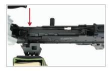
**Step 4.** Place the wire around the front of the gearbox and to the rear to plug in the power wire. Gently lower and close the feed tray parts and do not pinch the wires.
