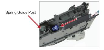
**Step 2.** Use the flathead driver to pry the spring guide post up. The phillips driver will then be slid through the back and center all the parts.
