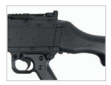
**Step 5.** When the stock is secure and the stock latch springs forward the top of the stock will be flush with the rear of the gun.
