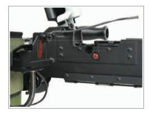
The curved spring transfers the BBs from the magazine to the hop up unit. The thin wire is to power the feeding motor in the magazine.
