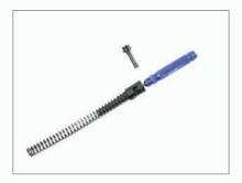
**Step 3.** Once the spring guide post is pulled up and out half way you can insert the phillips driver and get better control of the spring guide.
