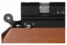
To activate the safety, push the safety catch lever rearward to the **S** position. When the safety is engaged, the trigger is locked and the rifle cannot be fired. To disengage the safety and fire the rifle, push the safety lever forward to the **F** position.
