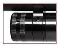
When charging is complete, bleed the excess air using the fill device bleed screw and remove the fill adapter from the rifle. When finished, replace the protective cover to prevent contamination of the fill port.
