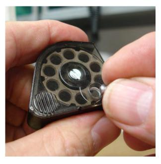
Load the pellets into the empty chambers
