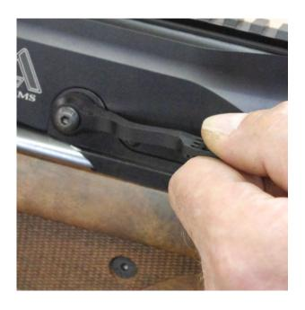
Close the lever to its starting position to lock the lever ready to fire.
