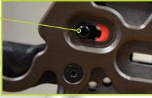
When the black post is all the way to the rear of the trigger box, it is on safe.
