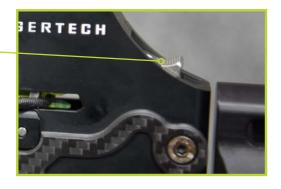
The white painted dot means it is on safe and the red painted dot means it is ready to fire.
