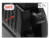
To lock the safety (put "ON SAFE"), press it in as shown in Fig. 2.a until it engages (red marking is not visible).
