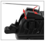
Loosen screw. Move sight sideways. Tighten screw.
