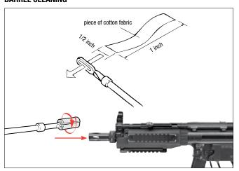
Put the safety ON SAFE and remove the magazine and the battery. Prepare a thin rod with a length of approx. 16 inches. Attach a piece of cotton fabric to its end and clean the barrel with some
