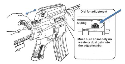
Pull the charging handle and open the ejection cover. Then you can see a hop up wheel inside as photo
