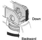
Use Calibrating tools to adjust the sight. Turning anti-clockwise to lowers the bullet hitting point or clockwise to higher the bullet hitting points
