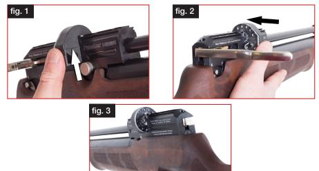
To load a pellet, push the side lever all the way forward as far as it will go.
