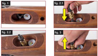
2) When charging is complete, bleed the excess air using the fill apparatus bleed screw. Once the line is bled, pull back on the fill adapter collar and remove the fill adapter from the rifle (fig. 3).
