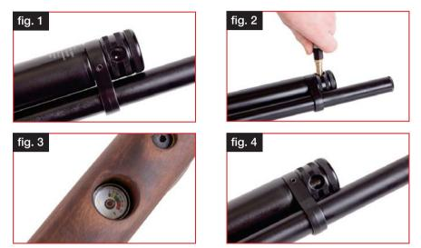
2) When charging is complete, bleed the excess air using the fill apparatus bleed screw and remove the fill adapter from the rifle. When finished, rotate the protective cover to prevent contamination of the fill port (fig. 4).
