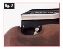
In addition to the safety catch, a loaded and cocked rifle can be made safe by decocking (uncocking). To decock the rifle, first pull the side lever back to the rear position and remove the magazine. While holding the side lever, squeeze the trigger and let the lever return forward under your control. The rifle is now decocked.
