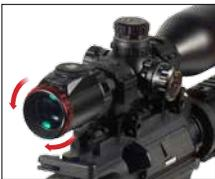
1. Diopter adjustment ring is located at the ocular end of the scope. Point the scope at an uncluttered and light colored background object, such as a white wall. Look through the scope and turn the dial ring clockwise or counter-clockwise until the reticle looks the sharpest to you at first glance.
