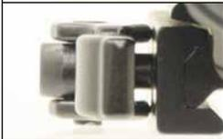
2. Turn the Cam Lever in the opposite direction to close the spring loaded locking plate, locking the QD mount base to the Picatinny rail.
