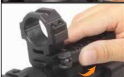
4. Should the Cam Lever not fully turn into the locked position and you feel heavy resistance, the locking plate tension is too high. Use the included Allen wrench to adjust the Hex Screw counterclockwise to decrease the locking plate tension by increasing the clamping width.
