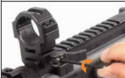
3. Should the QD mount base be loose, unlock the Cam Lever and use the included Allen Wrench to adjust the Hex Screw found within the Cam Lever Housing. Turning the Hex Screw clockwise will increase the locking plate tension by decreasing the clamping width.
