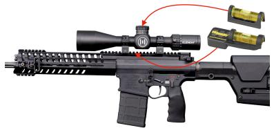
5) Once you are happy with the position of your riflescope, begin to torque down your rings in a criss-cross pattern, moving between screws and turning small amounts at a time. This will ensure that the riflescope does not shift position while tightening.
