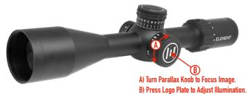
Tip: Place your riflescope in a fixed position and change the position of your eye (up/down, left/right) while adjusting parallax. If parallax is not set correctly, there will be apparent movement of the reticle in relation to the target. Adjust the parallax until this movement is eliminated.
