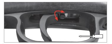
Turning clockwise decreases trigger travel Turning counter clockwise increases trigger travel.
