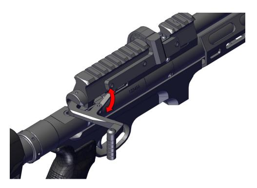
Note: It is very important that the cocking lever is pulled back to the correct position in one positive motion. The magazine indexes to the next pellet position as the bolt is retracted and it is possible for a partial index if the lever is not pulled back fully.
