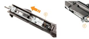
**Removing Bolt:** Press rearward on the loading nozzle (**D**) to separate it from the chamber and begin pushing the bolt from the upper receiver. Once the end of the bolt reaches the rear of the upper receiver, the bolt can be grabbed from the rear and pulled completely from the upper receiver.
