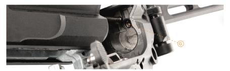
**Reinstalling Upper:** Align the recoil spring guide with the receptacle **(G)** in the back of the upper receiver and then slowly allow the rear lug of upper receiver to seat down into the lower receiver. Pivot the front of the upper receiver down so that the front lug aligns with the lower receiver. Once the pivot and takedown pin holes are aligned, push the pins back through the receiver until fully seated. Cycle the charging handle to ensure the bolt functions properly after reassembly.
