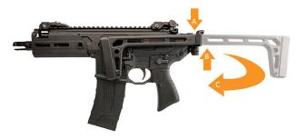
The stock can be folded by grasping the stock near the hinge and, while pressing against the top of the hinge (A), squeeze the stock upwards towards the hinge to unlock it (B). While doing so, pivot the stock to the left to fold it against the receiver (C). To unfold the stock, pivot the stock away from the receiver until it locks in the extended position.
