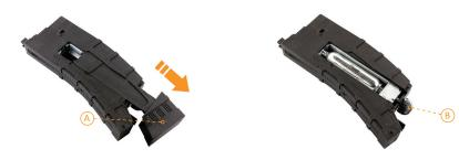
Press the magazine release button to remove the magazine from the airgun. Pull down on the bottom rear corner of the magazine (A) to remove the cover. Loosen the screw on the bottom of the magazine (B) before inserting the 12g CO2 cartridge into the cavity as shown. Then, tighten the screw on the bottom of the magazine. The sound of gas escaping will be heard as the seal is pierced. Continue tightening the screw until snug, then give one final 1/4 turn.
