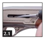
3 - Insert the cocking bolt and line up the screw hole in the bolt with the screw hole in the hammer. With the included allen key, install the allen head screw. Tighten securely.
