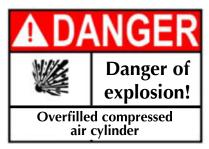
Do NOT exceed <u>maximum fill pressure</u> of 206 bar/3000 psi at room temperature!
