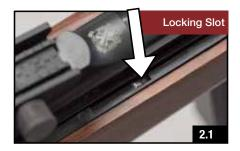
Once the pin is in the slot, the bolt will be held in the open position (Fig. 2.2). To release the bolt, pull back on the charging handle slightly and release it.
