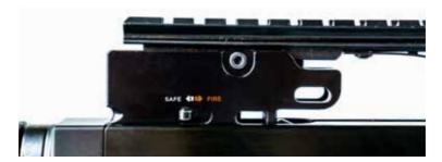
Figure 15: Trigger Safety operaton—Back siade SAFE front side FIRE
