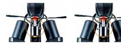
Figure 14: Cocking safety - left side: UNLOCKED / right side: SAFE or LOCKED
