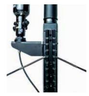
Figure 16: The string should be centered in the latch
