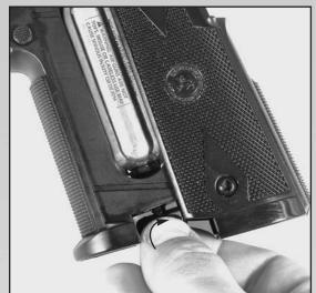
Screw the bottom of the compartment. When pressure starts increasing in the compartment (expansion of the CO2 in the compartment can be heard), finishing screwing rapidly. Very important: do not tighten excessively, it could permanently damage the O'rings.
