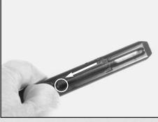
• Pull down the spring with the release. Fill the magazine with the appropriate 4,5 mm Steel BBs as shown. Maximum capacity is 20 BBs.
