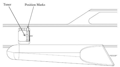
To increase tuner tension rotate it downwards, to decrease tension rotate it upwards. Increasing tension can help achieve higher velocities for light-weight projectiles.
