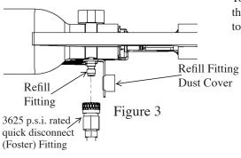
To refill your Spin-Loc Tank, attach the 3625 p.s.i. rated quick disconnect to the refill fitting. See FIGURE 3. A WARNING: BEFORE LOADING YOUR AIRGUN, MAKE SURE THE SAFETY IS IN THE ON SAFE POSITION AND THE MUZZLE IS POINTED IN A SAFE DIRECTION.
