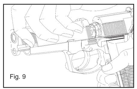
• The release lever must be in the horizontal position to lock the slide closed.
