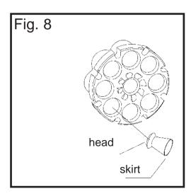
Remove the pellet clip and load the pellets head first (see Fig. 8) into the clip insuring that each pellet is completely inserted.
