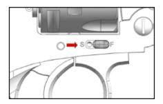
When you are ready to fire the safety catch can be pushed into the forward (fire position) with your right forefinger
