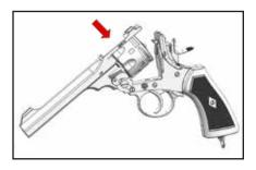
When all chambers are loaded close the barrel making sure that the barrel catch is in the fully locked position
