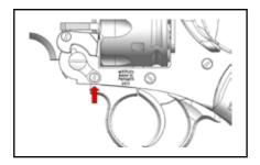
The revolver can field stripped by removing the screw indicated and rotating the cylinder cam lever anticlockwise, when the barrel is opened
