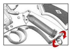
Turn the lanyard swivel clockwise to charge the  $\text{CO}_2$  capsule Then replace the left hand pistol grip
