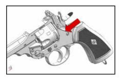
Push the barrel catch forward to open the breech
