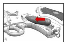
Load the CO<sub>2</sub> capsule into the CO<sub>2</sub> compartment
