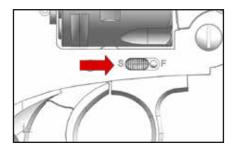
When handling the air pistol the safety catch should always be in the safe position towards the "S".
