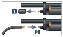
Remove the protective cap 1 and connect your charging equipment to the intake valve
