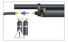
**4. Scuba tank**: Before disconnecting the hose from the rifle, bleed the hose gently and completely by allowing any residual pressure to escape. Then remove the filling equipment from the rifle.
