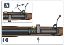
5. Pull the cocking lever backward to its open position until a click sound is heard **A** and slide the Twin-Shot-Tray into the opposite position **B**.
