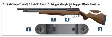
Note: To adjust the trigger, use a hexagon key SW 1.5 and a hexagon key SW 2.
