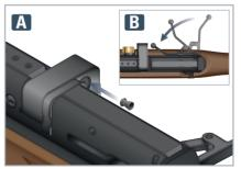
**6.** Insert a pellet flush into the empty loading opening of the Twin-Shot-Tray **A** and close the cocking lever **B**.
