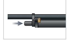
**5.** Put the protective cap back on the connector and screw it tightly.
