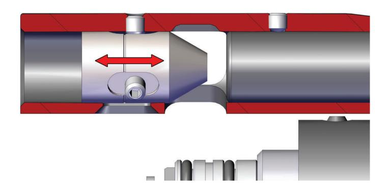
The factory set position of the cone is 4 mm. This distance has been chosen as a good starting position for most pellets. Note - This distance was the result of testing under factory conditions and may not be the best position in every case.
