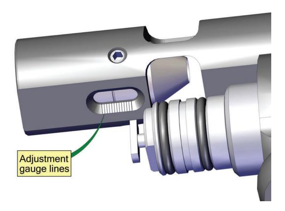
2. Loosen the 3 set screws holding the cone in position using a 2 mm allen key. Loosen these screws only enough to allow the cone to slide.
