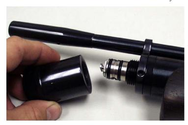
This is achieved by unscrewing the cover in an anti-clockwise direction.
