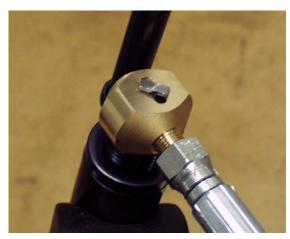
It is a wise precaution to hold the female part of the connector, during the filling procedure, as shown in the pictures below. This will ensure the female adaptor is located completely over the male part and prevent any accidental dislodging of the connector before you start to refill the cylinder.
