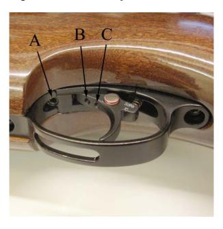
This rifle is fitted with a manual safety button located in the trigger blade.
