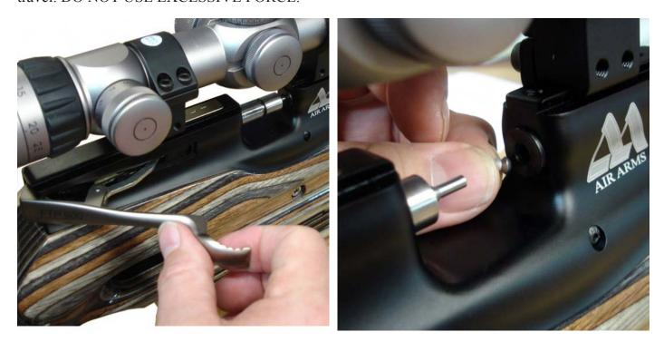
If the rifle does not cock, this may be due to incorrect trigger adjustment. The trigger also requires a pull through motion. If the trigger has not been 'pulled through' the sears may not have reset and will not be able to engage when the rifle is next cocked.
