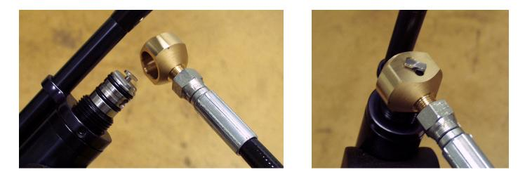
It is a wise precaution to hold the female part of the connector, during the filling procedure, as shown in the pictures below. This will ensure the female adaptor is located completely over the male part and prevent any accidental dislodging of the connector before you start to refill the cylinder.
