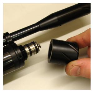
*This is achieved by unscrewing the cover in an anti-clockwise direction.*
