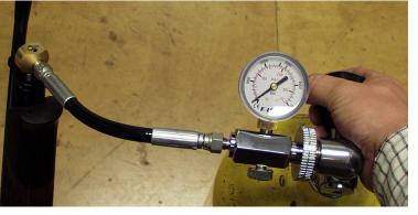
reached, close the valve on the bottle or stop pumping, open the bleed valve on the filling kit (to vent the hose, if you do not vent the hose you will not be able to remove the female from the rifle). Now the female connector can be removed from the rifle and end cap (E483BK) can be replaced over the male connector ensuring not to over-tighten.
