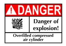
Do NOT exceed <u>maximum fill</u> <u>pressure</u> of <u>310 bar/4,500 psi</u> at room temperature!
