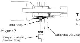
To refill your Spin-Loc Tank, attach the 3000 p.s.i. rated quick disconnect to the refill fitting. See FIGURE 3.
