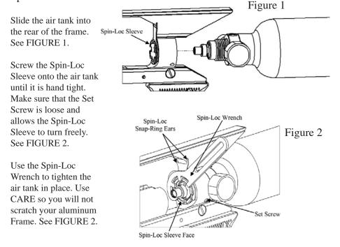
NOTE: If you have a Quick-Detach Air Tank, without the gauge and refill fitting, tighten the set screw to keep the Spin-Lock Sleeve from turning. Then screw in your Quick-Detach Tank as you normally do in a standard frame.
