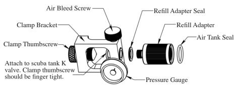
If you fill from a scuba tank that has a K-valve, the AirForce refill clamp is the way to connect your air tank. The square clamp attaches to the K-valve and mates with the O-ring in the scuba tank valve. Once the refill clamp is attached to the scuba tank, close the bleed screw and screw the air tank into the adapter.
